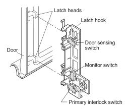
Figure C-1. Latch Switch Adjustments
